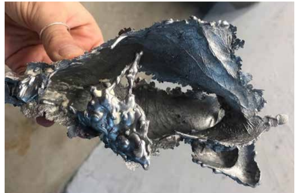
First pieces casted in aluminum using the investment technic.
