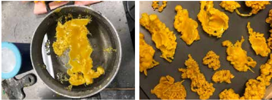
Process and results of shaping the melted wax in the cold water.
