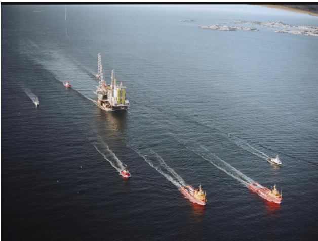
Towing the Troll-platform from Stord (1995), Photo : Bjørn Østrem, National Library .
