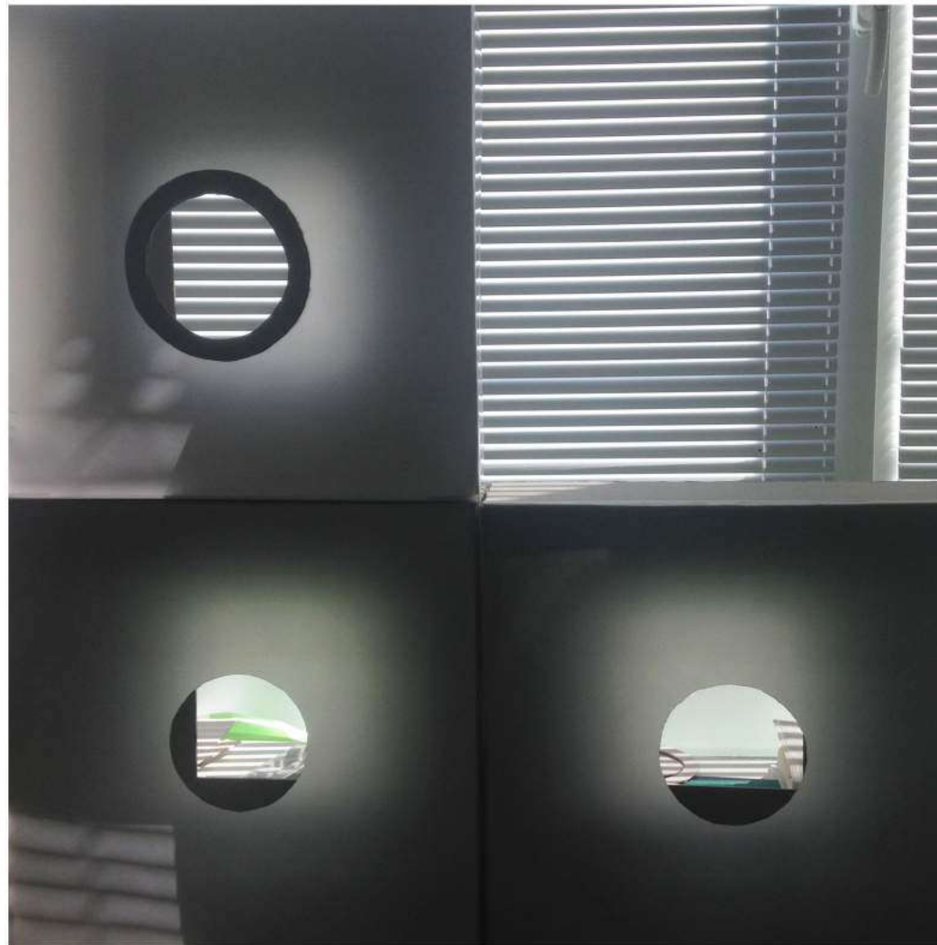
Figure 15. 30 x 30 cm boxes made out of chipboard with screens made out of vellum paper
