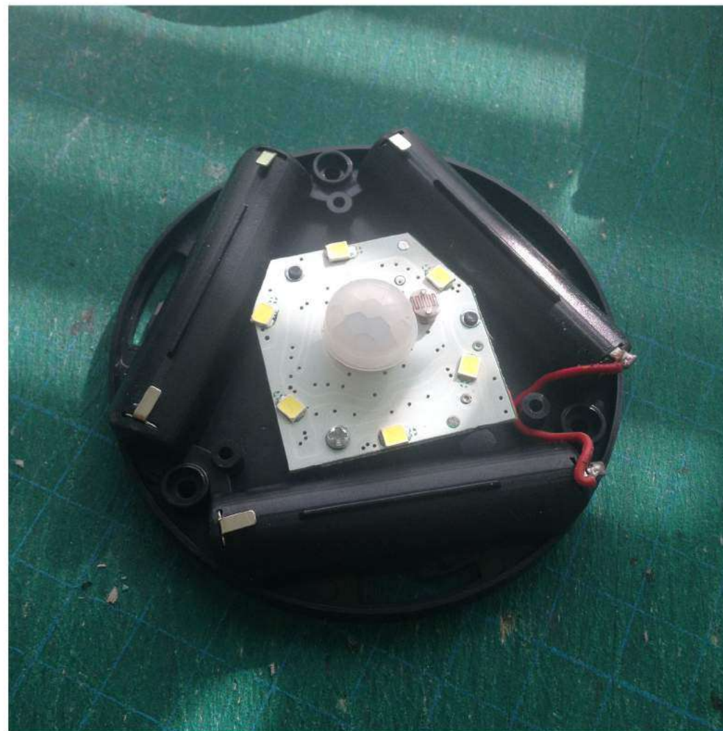
Figure 18. "Unhoused" puck light with 6 LED lights exposed
