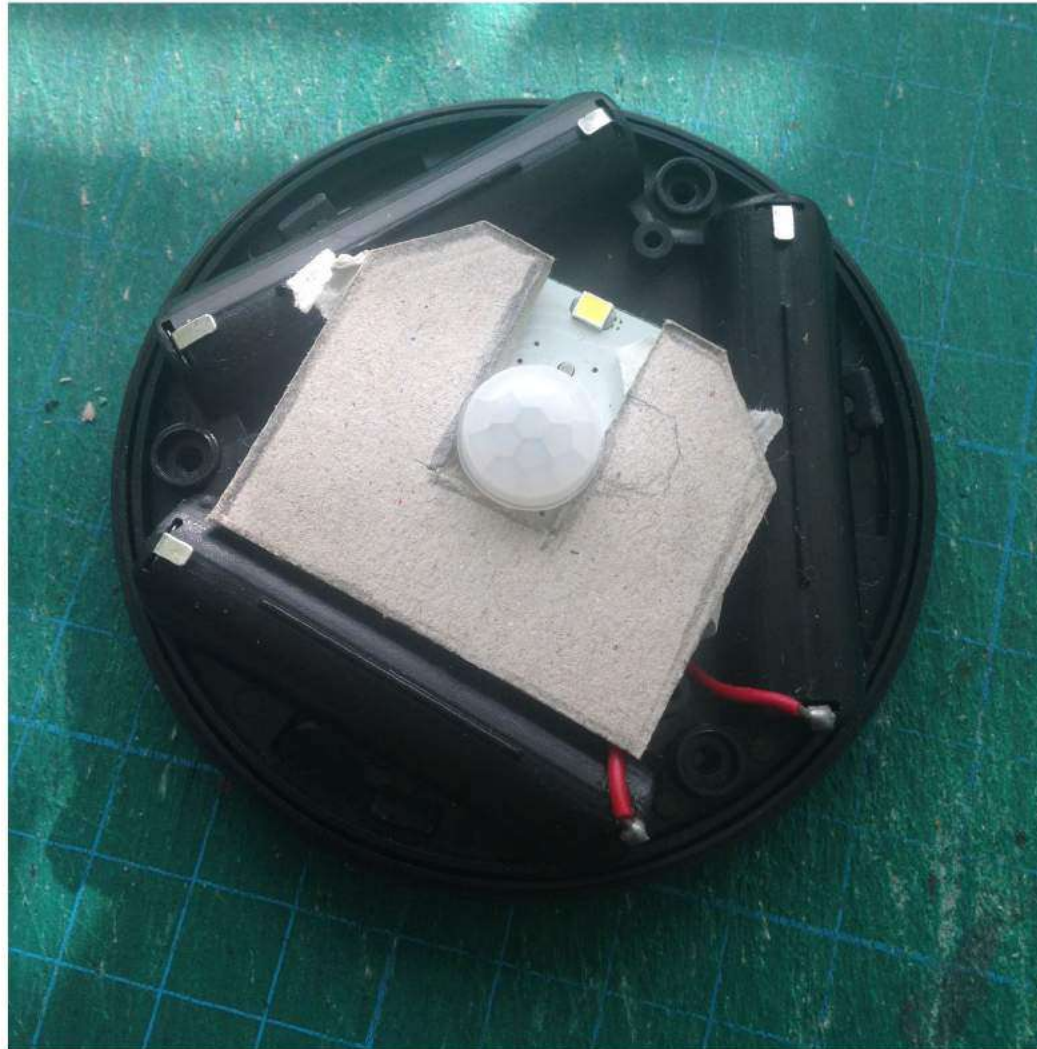
Figure 20. "Unhoused" puck light with makeshift "lightblocker" concealing 5 LED lights and exposing only one single light source.
