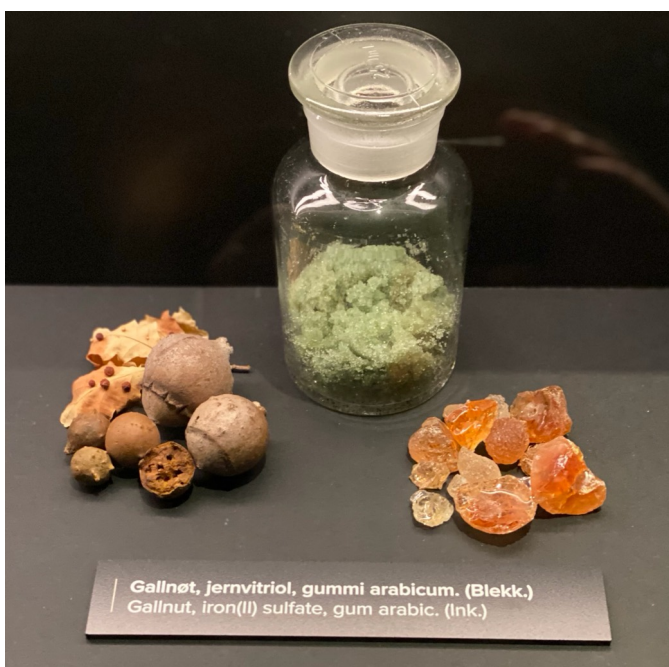
Fig. 3—the ingredients of ink in colourful display: gallnut, iron(II) sulphate, gum arabic.
