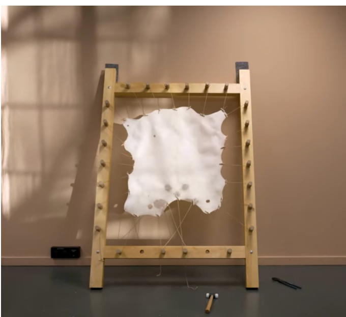
Fig. 2—A skin stretched for scraping and smoothed with pumice stone, in the making process of a parchment. It would take approximately 200 sheep skins to make a Bible. Before Gutenberg (paper and press) a bible took toll of a considerable livestock of sheep.
