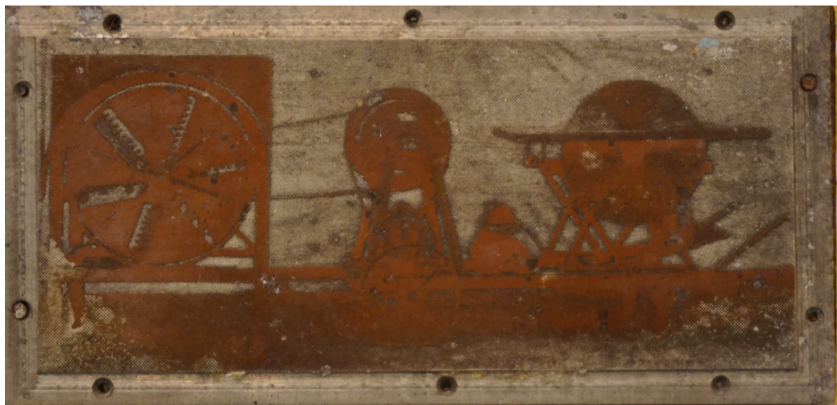
Here is an example of a relief printing plate used in typography. The photographic emulsion is still on the surface. Photo Jan Pettersson
