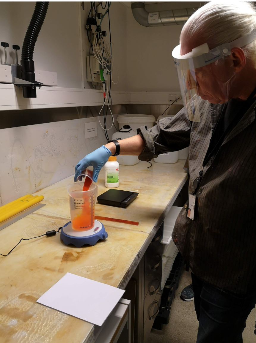
Working with the Photogravure club at Oslo National Academy of the Arts Department of Print Mixing the Dichromat solution for sensitizing the pigment paper
