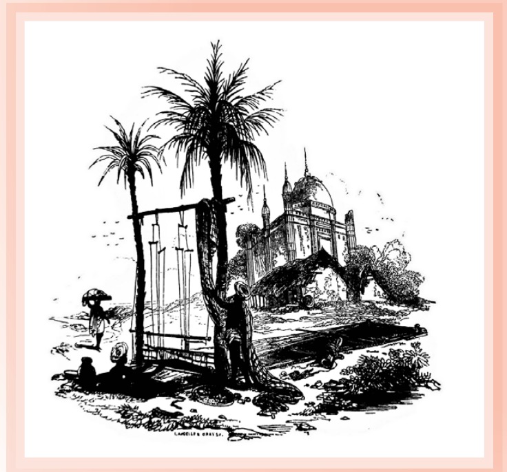
Indian pit loom (1835). The weaver sits in a pit in the ground with the warp suspended out on ground level, solving the technical problem of building an outside structure. The shafts are using palm trees as supports.
