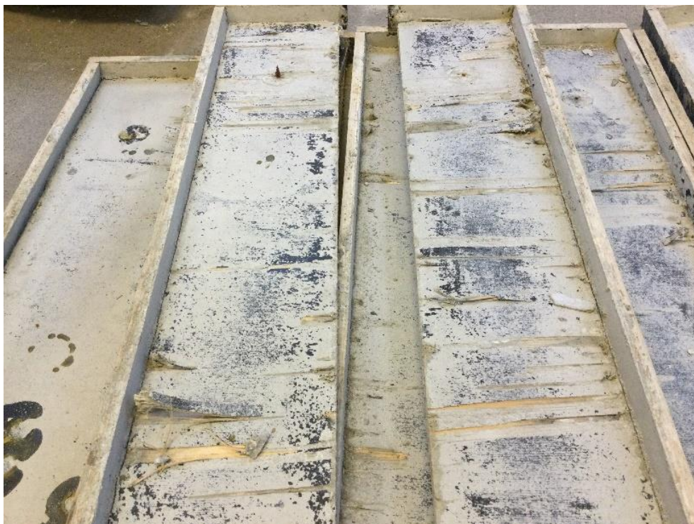
Image28- Example of wood casting moulds and the deterioration from the extreme amount of use.
