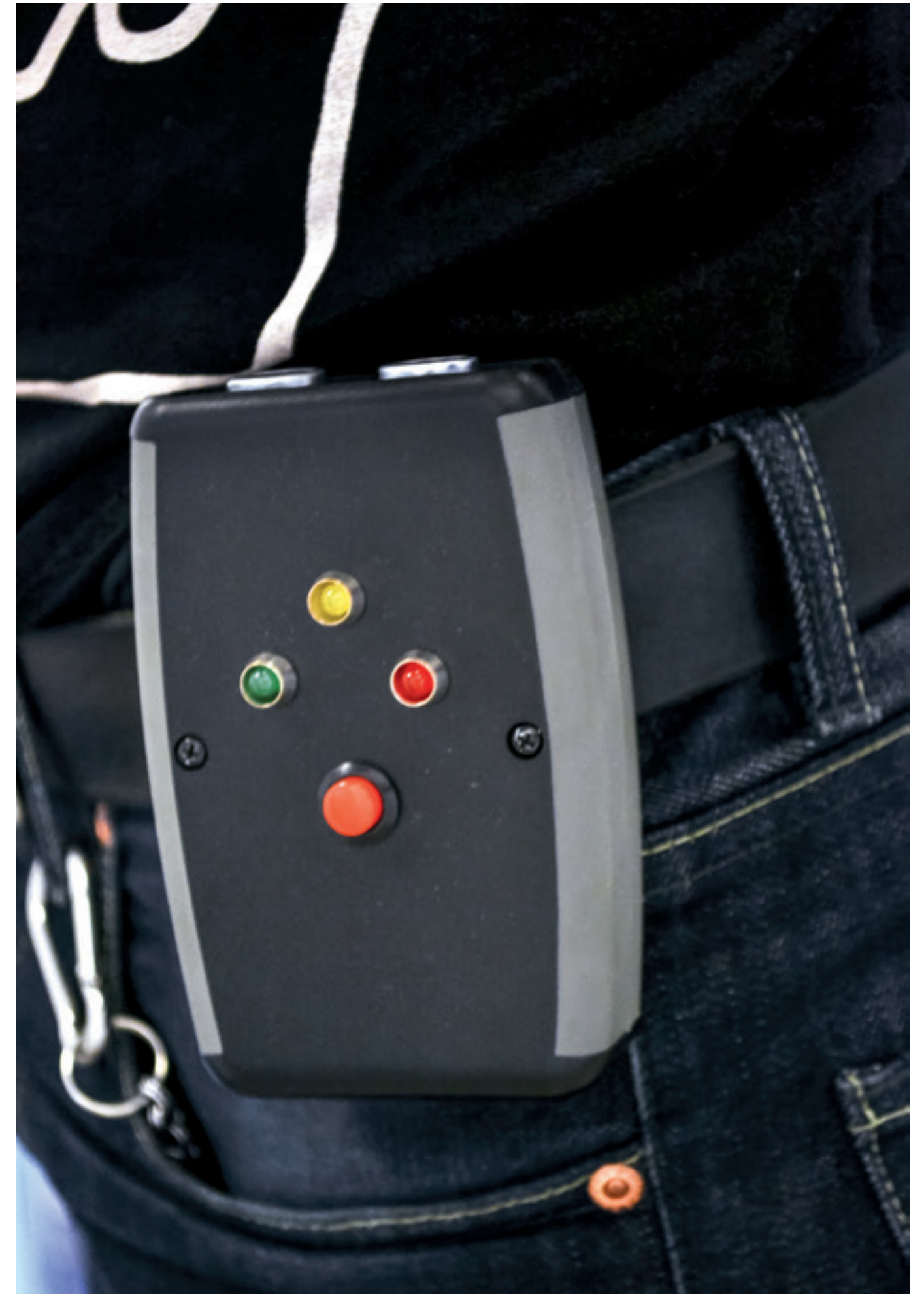
Conversation Distance Meter 2015, electronics case, battery, LEDs, ultrasonic range finder, microchip, steel, 8 × 12 × 5 cm.
