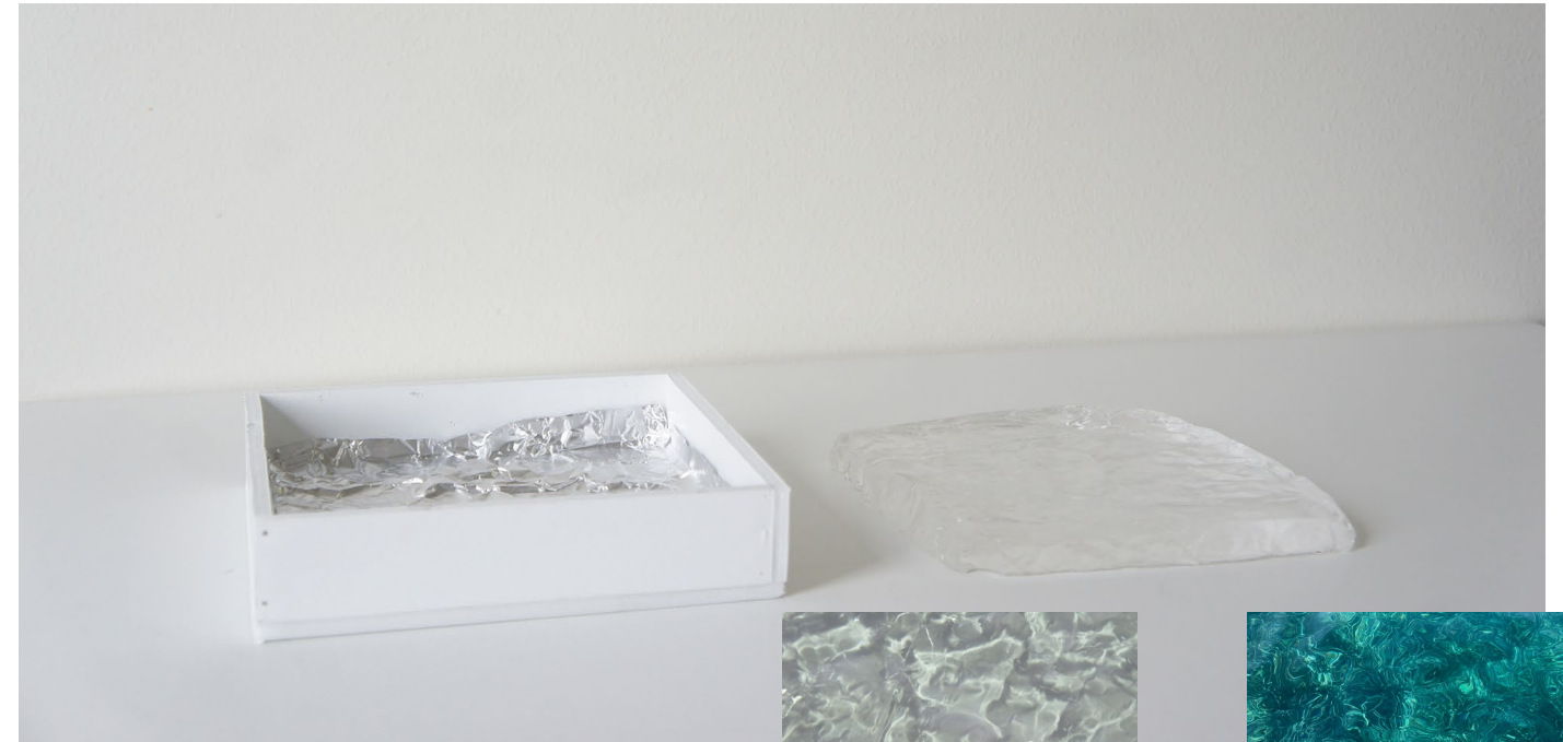
Sample of silicone (160mmx160mm) molded in a cardboard covered with crinkled aluminium papersquare
