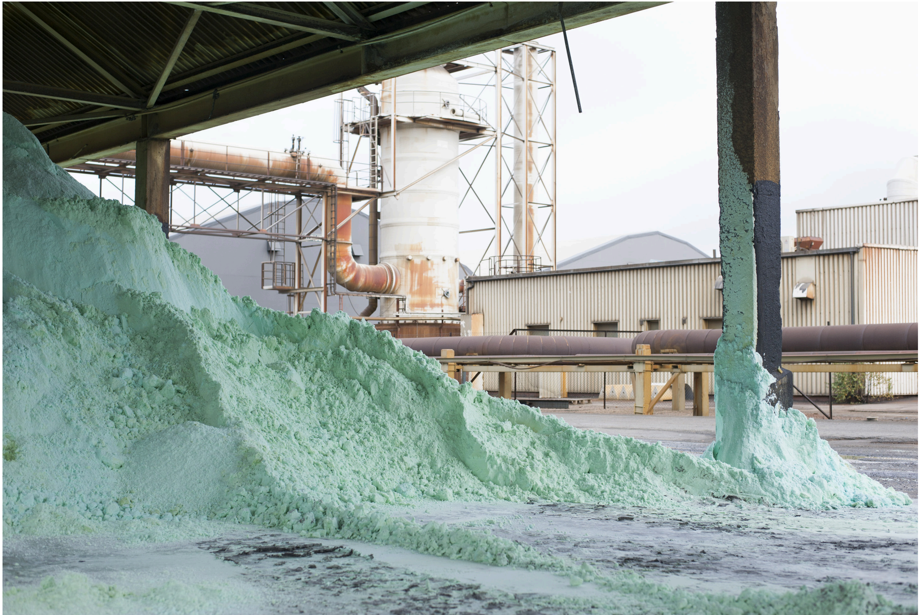
Iron sulphate deposit at the titanium dioxide factory Kronos Titan AS, Fredrikstad
