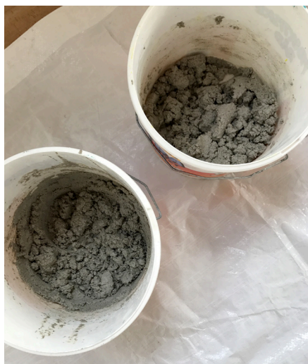
Coarse and fine lime plaster for fresco
