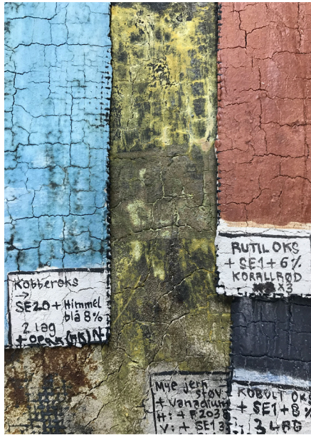
Ceramic glaze tests with various oxides
