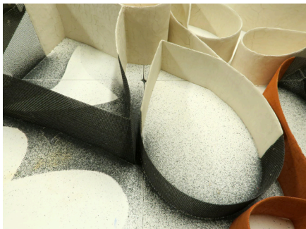
Steel-reinforced ceramics after firing
