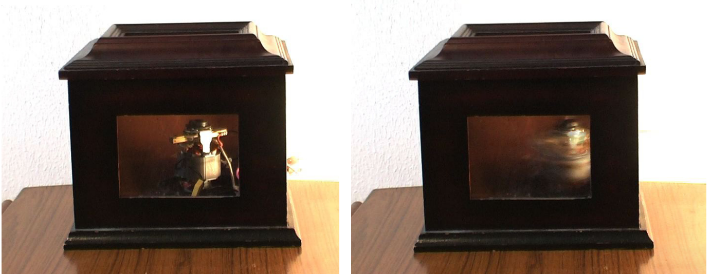
Vacuum cleaner engine inside wooden box
